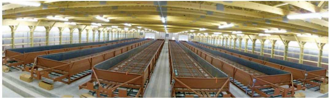
RT Solutions in Avon, New York recently expanded its vermicomposting capacity (above). Raw cow manure solids are mixed with chopped silage and precomposted prior to being fed to the worms in a 1- to 2-inch layer on the top of the beds.
